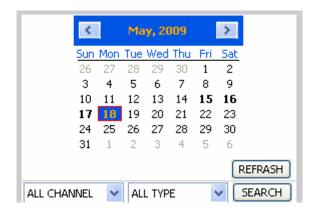
The highlighted date indicates video was recorded on that day. RED FRAME means the date is system date, click the date will search that days' recording file list. For example, the above picture display 2008, Dec. 3rd,4th,5th,6th,8th,9th,10th,11th,12th,17th,18th have recorded video, and system date is 18th, Dec, 2008, current search date is 17th, Dec.
