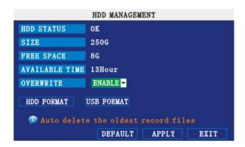
**HDD STATUS:** There are three status available, normal, un-format, No HDD. If HDD cannot run normally (including unformatted and no HDD), there will be a 【H】 displayed on video live view.
