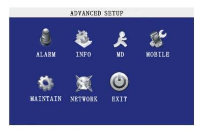
Advanced Function includes Alarm settings, system information, Motion detection, mobile phone monitoring, system maintenance and network setting.
