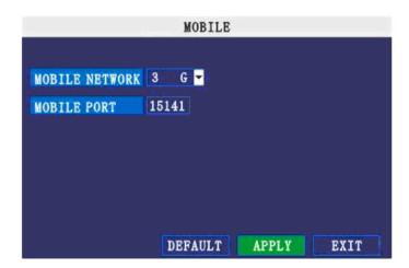
**MOBILE NETWORK:** Select different mobile network from the options of 3G, 2.5G and 2.75G; press [APPLY] to choose different network.
