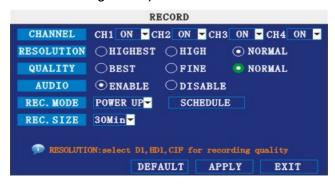
CHANNEL: ON: Means the channel is enabled to record
