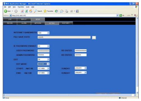
**BANDWIDTH:** Set the bandwidth in kbps (128k、192k、256k、384k、512k、1024k) that you want to allocate for traffic that matches the internet. This bandwidth does not include audio.
