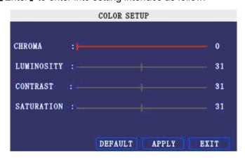
Press [Enter] or [+] [-] key or directly drag the cursor to setup colors, including chroma, brightness, contrast and saturation, press [APPLY] to save the parameters once the setup is completed.
