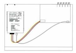
3) Affix HDD on HDD plate as indicated below with the screws.
