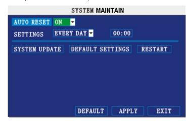
AUTO RESET: When it is on, you can setup the time for device to restart.
