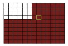
Press the direction key on remote control to move cursor along the small pane: position of cursor is indicated by green frame. Press 【Enter】 to select or cancel motion detection of this small pane. When setup is finished, press 【exit】 to go back to MD setup interface and settings will be saved automatically
