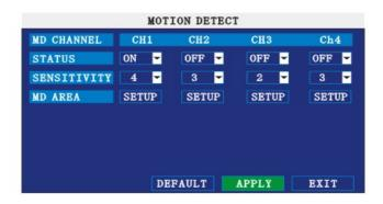
**STATUS:** Each channel has corresponding channel switch, press 【Enter】 to turn on or turn off the motion detection for each channel.
